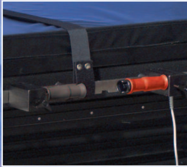
Push button (on red handle) releases tabletop for free-float X-Y motion.
